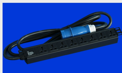
8-outlet All-usage PDU, 2P+E industrial plug 32A input, 10A all usage outlet, without switch, with 3.0m length cable, 19" positive installation with TOTEN logo (322000796)
