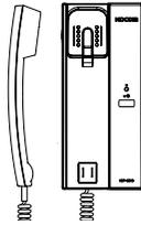
Pick up the handset and communicate with a visitor. After end of communication, return the handset where it is locked.
