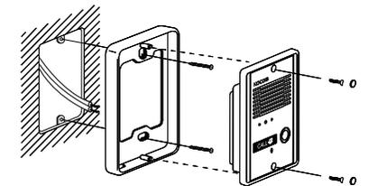
After attaching the body supporter with 2screws, put the indoorstation into the grooves of body supporter, and then fix it with screws.
